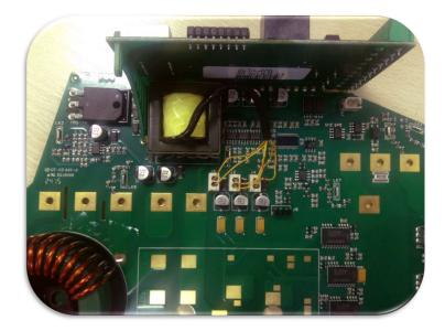
With the heatsink removed, access can now be made to the IGBT module
