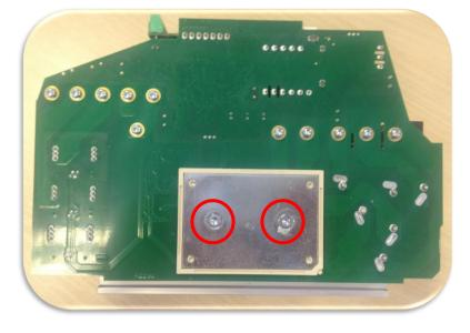
Using a torx T20 screwdriver remove the 2 x screws holding the IGBT module (2Nm) (highlighted in red)
