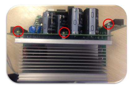
Using a torx T20 screwdriver remove the 3 x ground pillar (1.5Nm)
