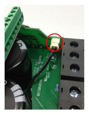
Depending on the HP rating a fan may be fitted to the drive. The fan connection is highlighted opposite.
